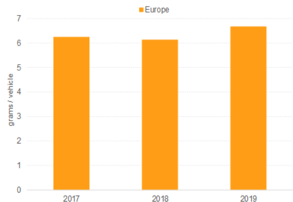
Figure 6: PGM loading per vehicle. Euro 6d Temp or RDE introduction increased PGM loadings in Europe in 2019, also offsetting some COVID-19 related demand loss
